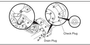
Fig. 31 Add, Check and Drain Rear Axle Lubricant
